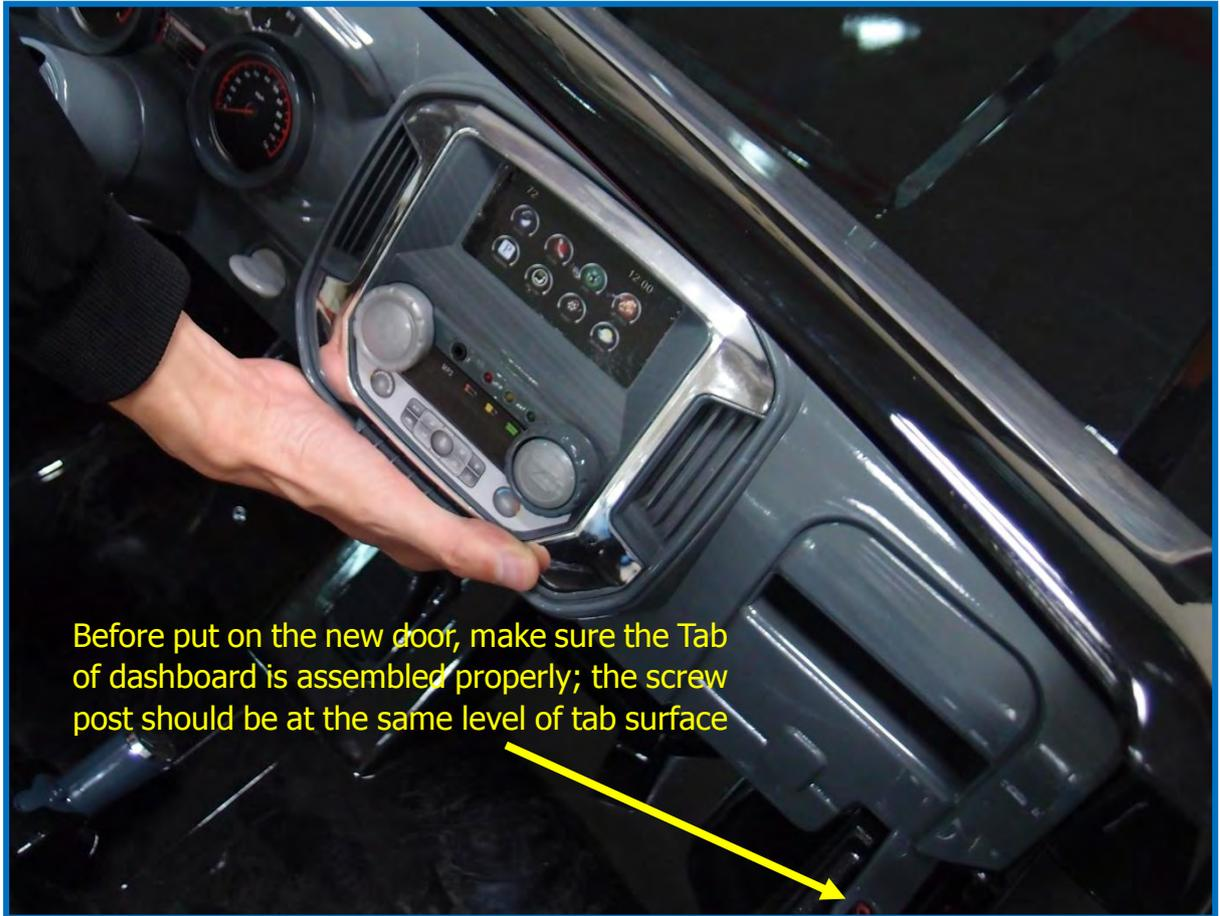
Before put on the new door, make sure the Tab of dashboard is assembled properly; the screw post should be at the same level of tab surface
