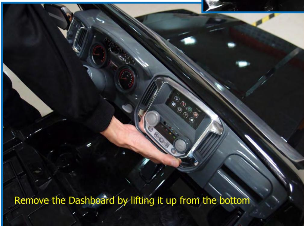
Remove the Dashboard by lifting it up from the bottom
