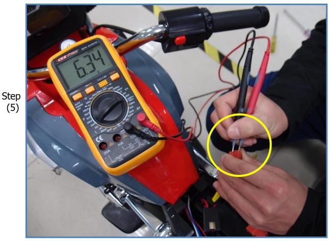
Reading Judgment:  $6.0 \text{ V} \sim 6.5 \text{ V} - \text{Good condition}$
