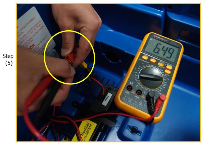
Reading Judgment:  $6.0 \text{ V} \sim 6.6 \text{ V} - \text{Good condition}$
