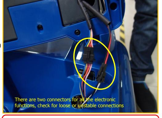
If problem is solved, reverse above steps to re-assemble the vehicle. If not, unplug the connectors and continue to check the wiring inside Dashboard.
