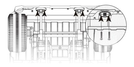
6. Turn over the truck body and align the holes and fasten the four screws (26) accordingly.
